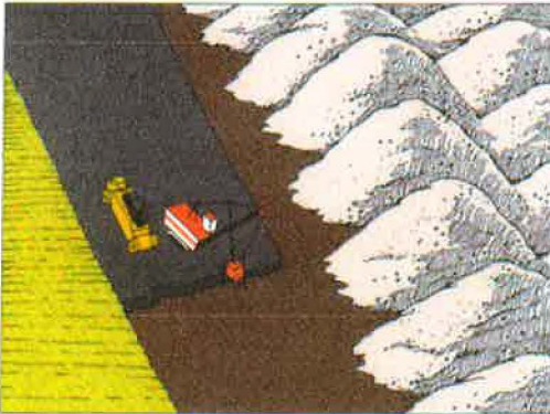
2. When the earth is removed, the lignite is dug out and loaded into haul trucks.
