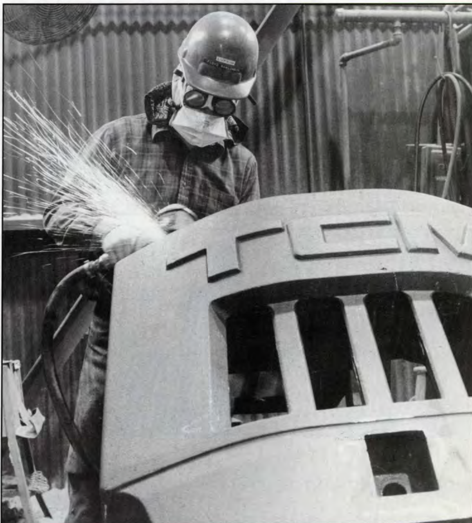
In the Cleaning Room, Floyd Rawlinson, Chipper-Grinder-Finisher, removes excess metal from an outside casting.
