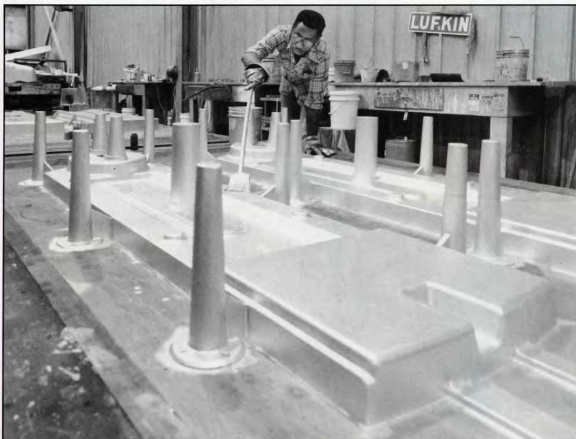
James Davis, Pattern Tender, applies a parting material which prevents sand from sticking to the pattern and allows easier separation from the mold.
