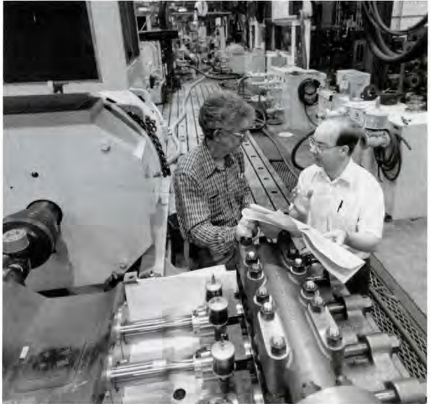
Electrical Designer Gene Hargis, left, discusses the procedures for testing the Ingersoll reciprocating pump with an Ingersoll employee.
