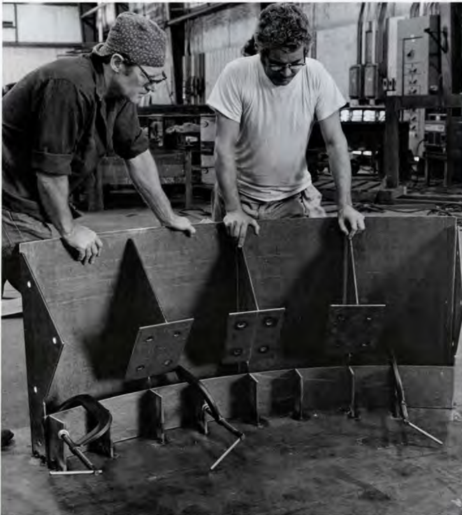
A partially assembled vein mill kit is clamped to a welding jig in the old structural shop. Welders Jack Kirkland and Andy Anderson inspect the unit.
