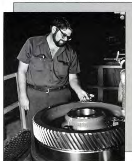
Ronnie Smith cuts teeth in a gear using the milling process.
