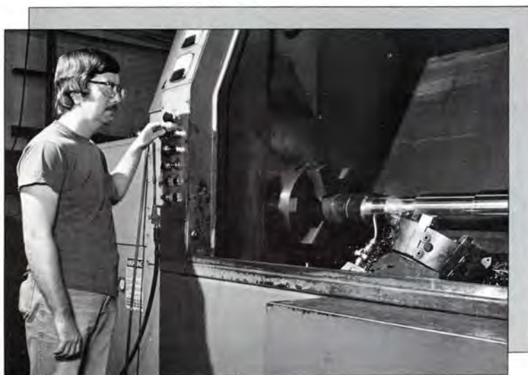
Larry Blanton operates a numerical-control lathe, utilizing the turning process to shape a high-speed pinion.
