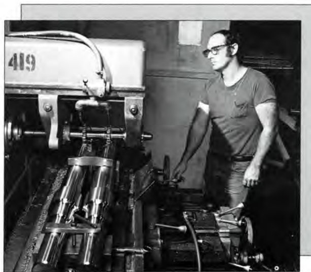
Ronny Parker runs a milling machine, shearing metal to cut a keyway in a pinion.
