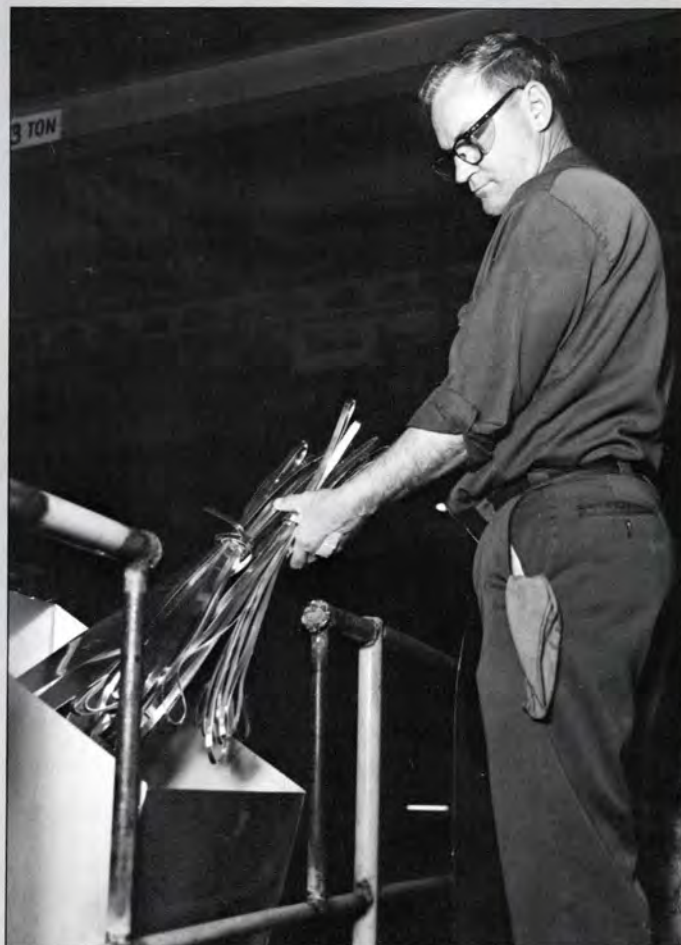
Charles Kendrick's, Trailer Division assembly foreman, tosses scrap down a metal chute, sending the scrap from the elevated platform to the shop floor. Kendrick suggested building the chute to reduce material handling --- one aspect of the MAX-2000 project.
