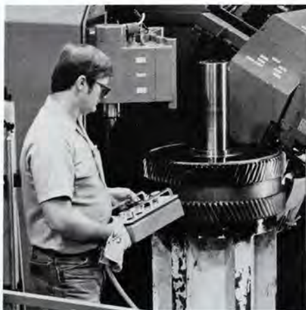
Victor Reese machinist, is operator of the latest Hofler Gear Grinder.
