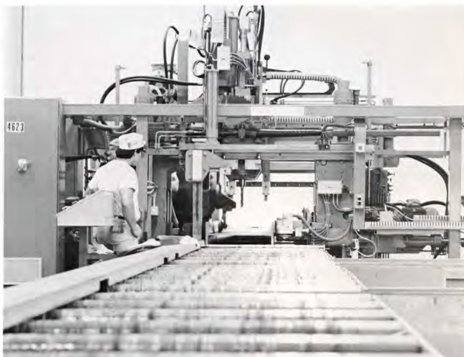
The structural plant's new Peddinghaus drill line was fully operational just days before the first beams for the baghouse facility were being produced. Here Jacob Marquez operates the Peddinghaus.
