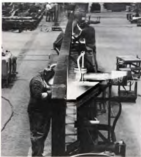
The biggest costs in the production of new lightweight platform trailers is in the fabrication of the trailer's two center beams. The beams with two transitions, from 11 inches down to 26 inches at the front and back up to 19 inches in the rear, require more fabrication work for LUFKIN employees.
