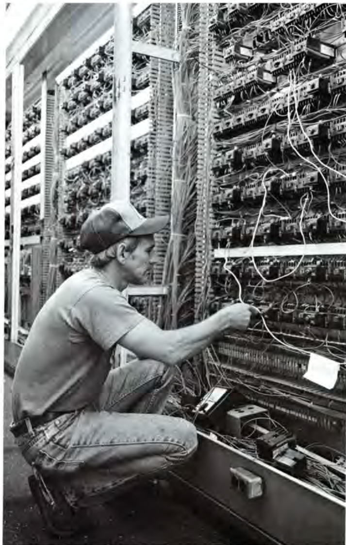
Trouble shooting problems in the giant control room of the trailer plant's Pierce-Rivet machine is Larry Havard, one of over 200 skilled maintenance mechanics throughout the company responsible for the upkeep of increasingly more complex, computer-controlled machines.
