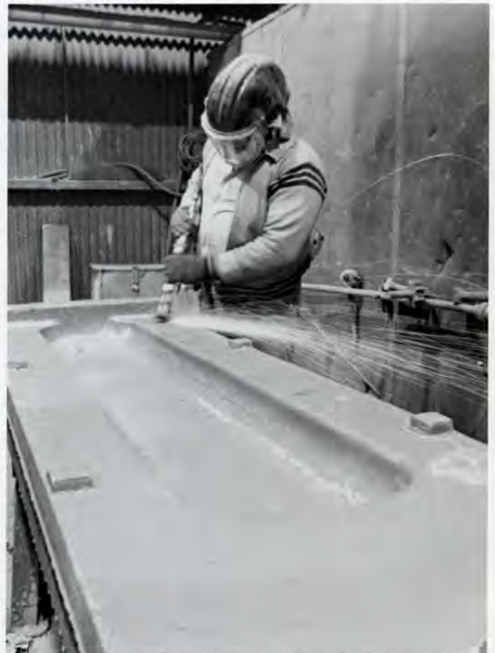
Thomas Jenkins, who insists he loves his work in the LUFKIN foundry cleaning room, is shown here operating a pneumatic grinder. He's well protected with a shielded safety helmet.
