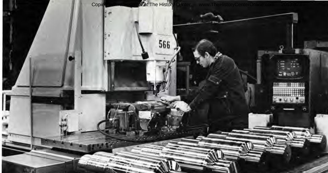
"We've always furnished our skilled workers with the finest tools of their trade," says company president Frank Stevenson. Here, production technician Jerry Wigley operates a $123,000 Milwaukee VB4 computerized vertical keyway machine that is used in the production of pumping unit pinions.
