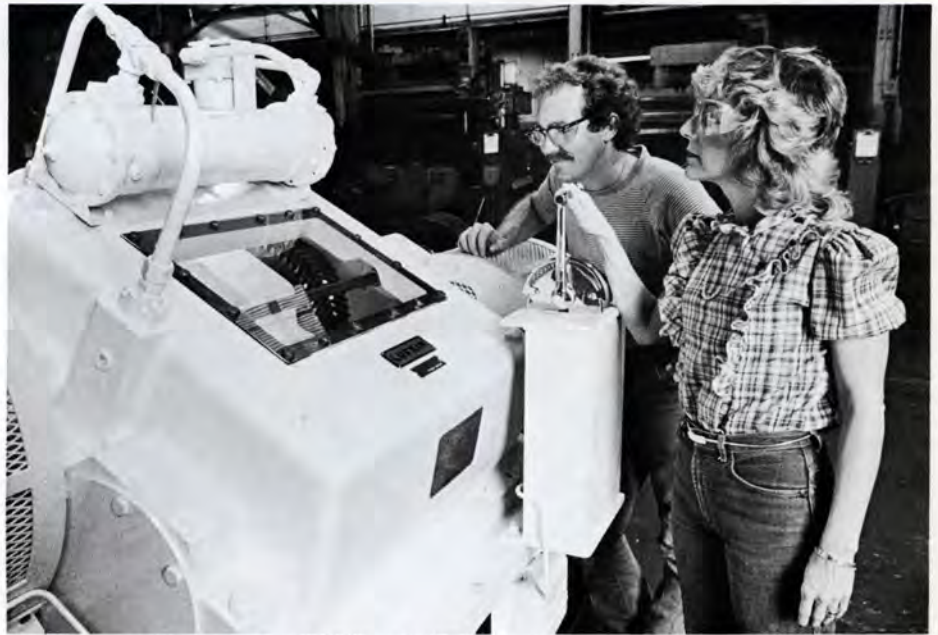
Pam Lovett, office services, and William Redd, Jr., material control, look over the new case-hardened and ground marine gear on display in the industrial gear machining area.
