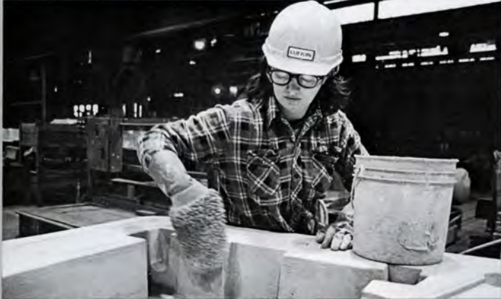
Nancy Ballenger demonstrates the mittens that she makes for applying mold washes to molds.
