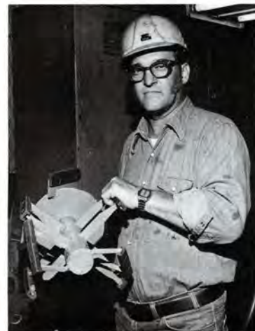
(Left) The no-bake machine in the main bay of the foundry blends sand, resin and catalyst together, and then pours it into the molds. Ferguson developed a new type of mixer head for this mixing process. (Above) Ferguson lined the mixer blades with a plastic-like substance called Tivar 88. The surface reduces the effect of abrasive action.
