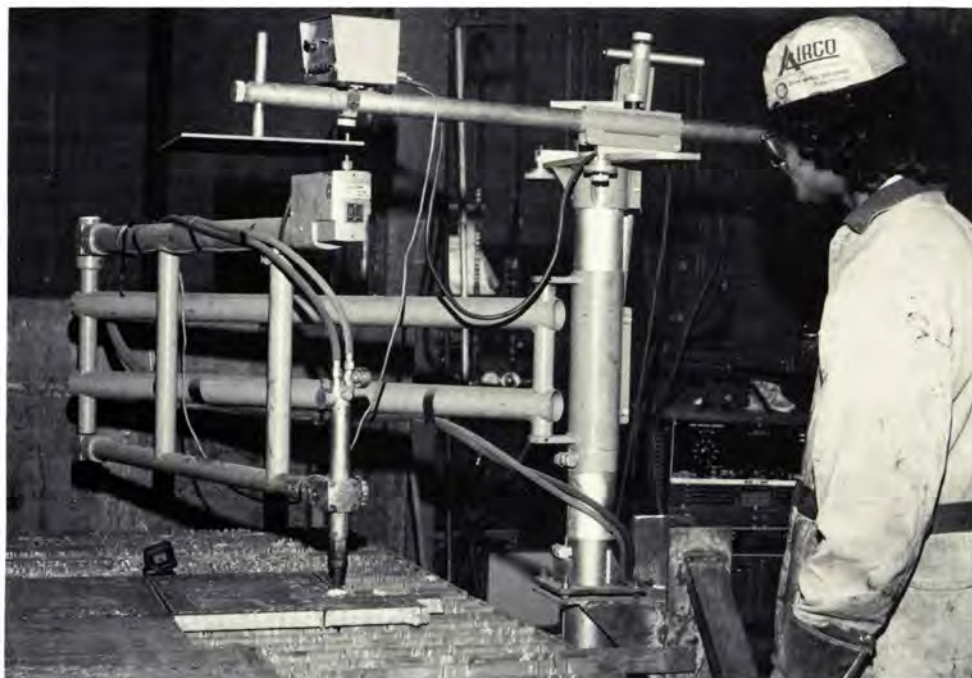
Jack Singh operates the plant's shape burner which is used to shape structures from patterns or templates. The machine was purchased from a firm in Colorado.
