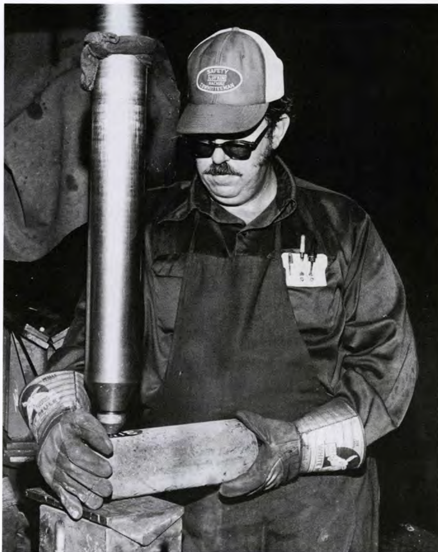
Charles Hodges is subjecting a component part to a Brinell test to determine its hardness. The machine makes a small indentation in the metal. The surface measurement of the indentation determines the degree of hardness.
