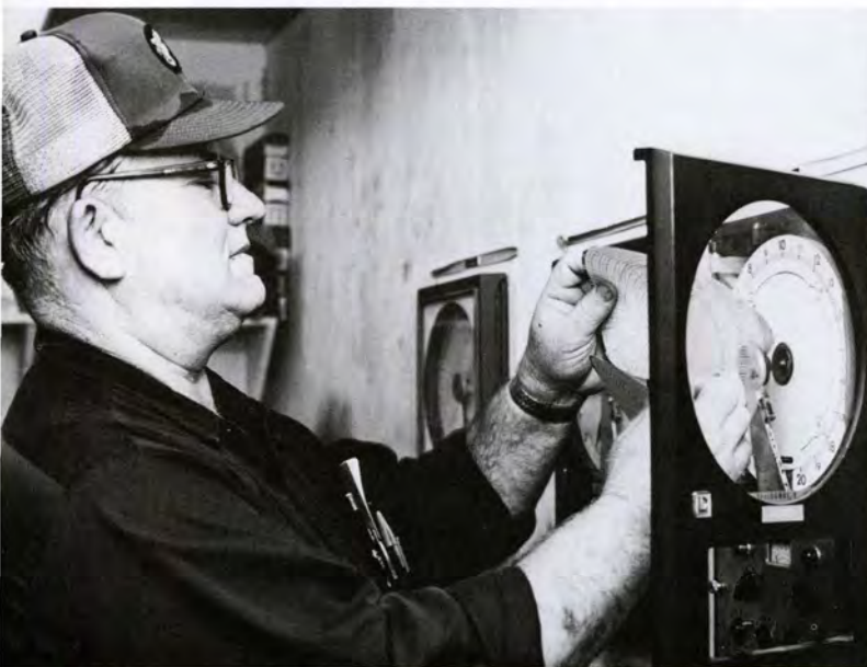
A. C. Lunsford, first shift foreman, checks the temperature and time on a load of parts in the furnace for heat treating. Records are maintained on every part that goes through the department for heat treating.
