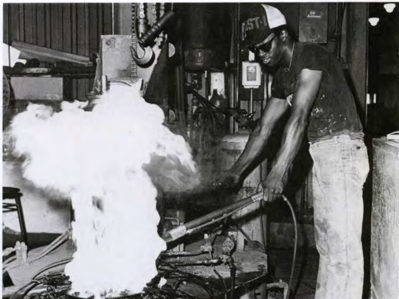
Parts which must withstand great pressures are often flame-hardened, a process that results in a thin layer of extremely hard metal on the exterior of the part. Here, Clarence Ray Newton, flame-hardens a shaft. Flames heat the steel while water jets rapidly cool the metal.
