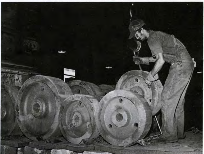
Gear blanks are loaded on a furnace car by Ronnie Garrison. These blanks will be baked overnight at temperatures of 1650 degrees and unloaded in the morning by the first shift crew.
