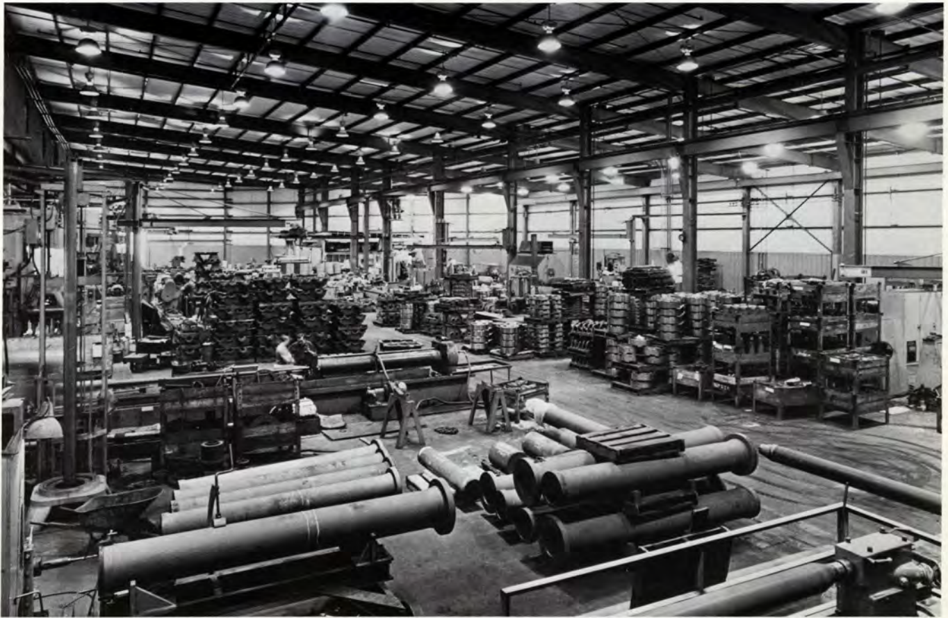
The new 37,000 square-foot extension to the machine shop houses machines that produce cylinders, gear housings, sheaves, brake drums, and gears. Construction on the new facility began in June, 1978.
