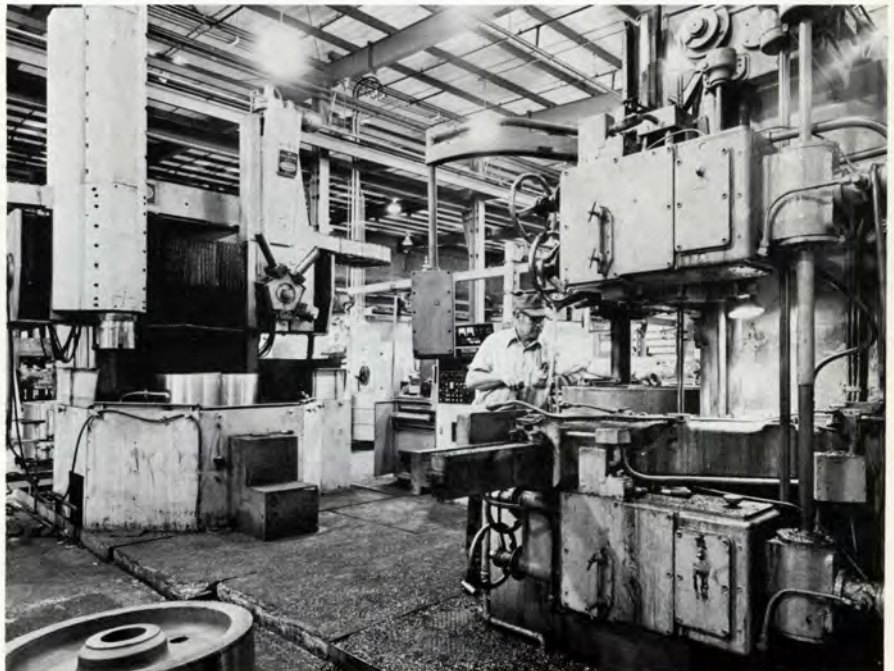
These two vertical turret lathes are known as a "work cell"—the numerically controlled machine on the left puts the finishing cuts on a gear blank after the manual machine, right, prepared the rough casting.
