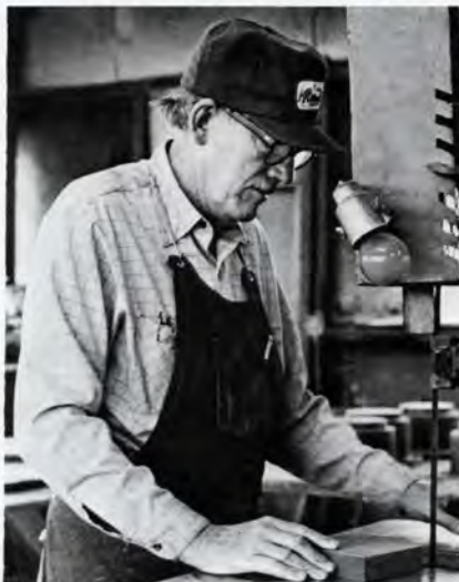
Maurice demonstrates a 100-year-old band saw which has been used by the foundry's pattern shop since 1909. The saw originally consisted of wooden pulleys driven by a motor, but because of the danger of fire, the pulleys were replaced with metal ones.
