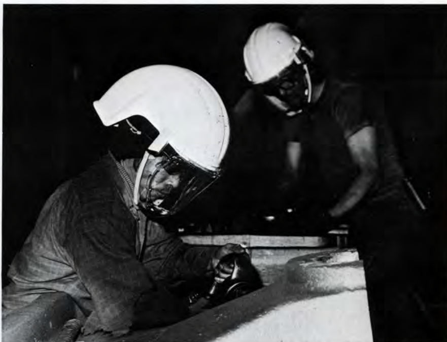
(l-r) Van Phuoc and R.R. Daniels, both cleaning room, 1st shift, wear the new Racal Airstream AH5 hoods now in use in the cleaning room. The hoods cost $300 each and feature respiratory, eye and face protection.
