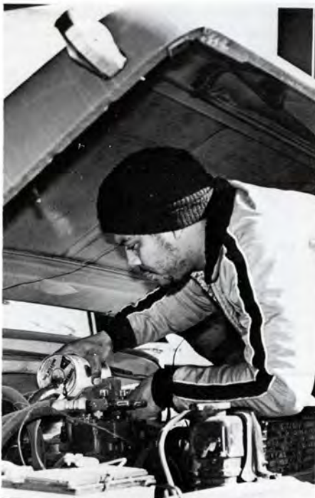
Robert Lewis adds a quart of oil to one of the company's trucks. Many of the truck-tractors can hold from 42 to 48 quarts of oil. Oil is bought in bulk from a local oil company and from LUFKIN's Automotive-Industrial Supplies Division.
