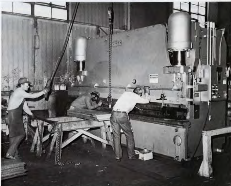
One of the year's largest expenditures in the structural shop was for a Pacific pressbreak machine. The machine reduces the time necessary to bend structural pieces by reducing the number of handlings
