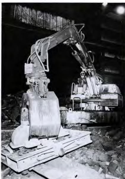
The new castings manipulator, one of two pieces of equipment specially designed to meet LUFKIN's needs, can reach 25 feet and lift 25,000 pounds. This speeds up removal of hot castings from shakeout station
