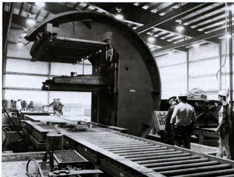
The new roll-over machine for the main bay foundry is the largest roll-over machine made, the first of only two machines ever built. According to Clayton Jircik, LUFKIN's need for such large equipment is unusual, "We're unusual in that we make so many large castings. Our castings are some of the largest produced anywhere."
