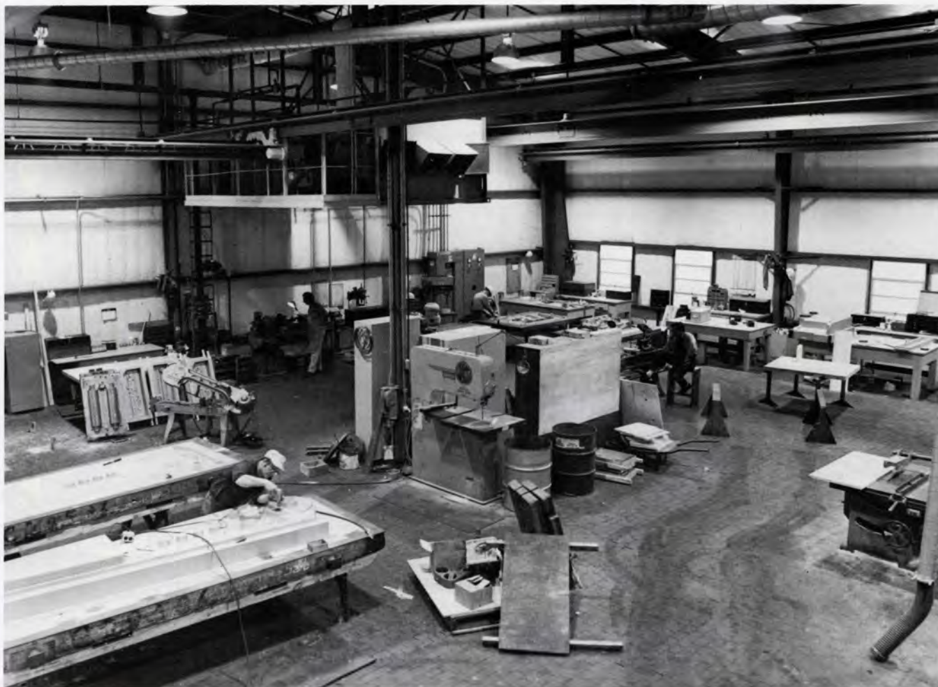
The new pattern shop is 2800-square-feet larger than the old building. In addition, the new building has two overhead cranes, a 2-ton and 3-ton, and larger work areas between machines which should improve work flow
