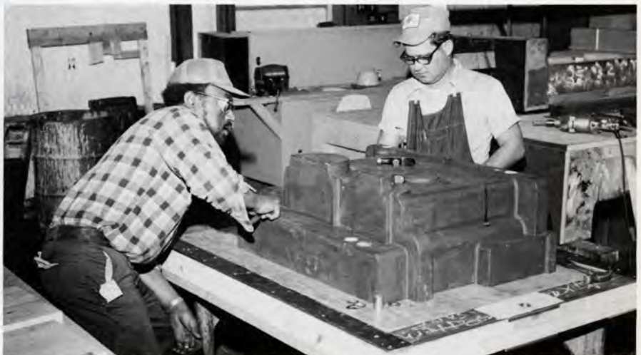
Willie Mitchell, left, and Floyd Boozer combine their talents to finish off a pattern. Patterns must be extremely accurate to make sure the molds and castings are up to LUFKIN quality
