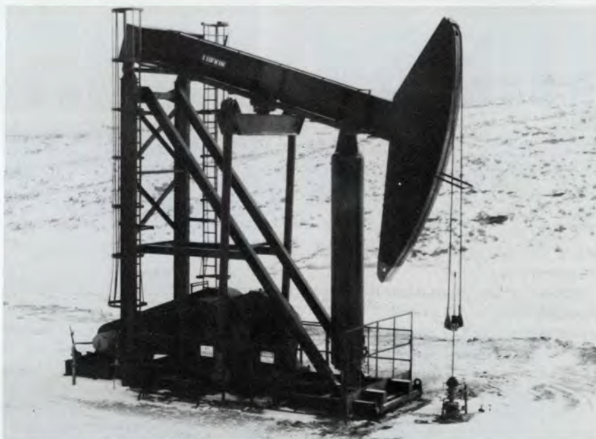
Continental Oil Company installed a LUFKIN air-balanced unit, A-2560D-470-240, on their Sussex-Tensleep B Well #192 the last week of December, 1977. This is the first time an air balanced unit of this size has been delivered to the Rocky Mountain area. The unit requires a 200-hp prime mover and has a maximum load on the wireline hanger of 40,000 pounds.
