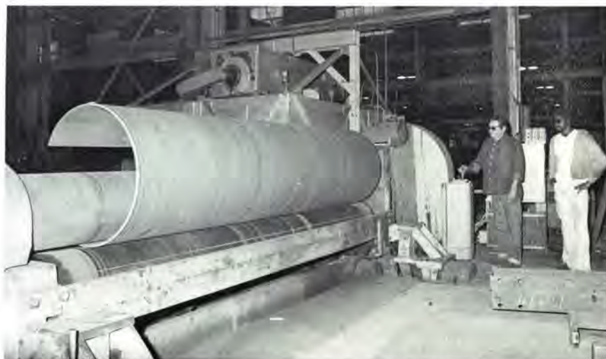
Bertsch plate roll machine rolls cylinders from flat plates to form tanks for air balanced units
