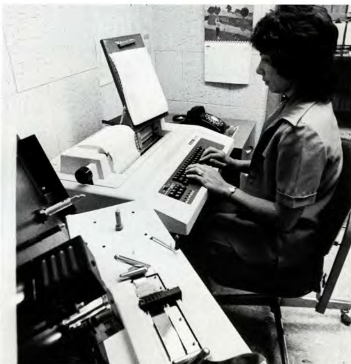
Jonell punches tapes on the new NC tape preparation machine called Numeridex. The NC tape preparation machine has limited computer like capabilities that allow the terminal to perform many functions. Before the addition of this machine, Jonell had to operate two machines: one to punch NC tapes manually and a teletype to transmit data to a computer based in Houston. The Numeridex performs all of these functions in one terminal
