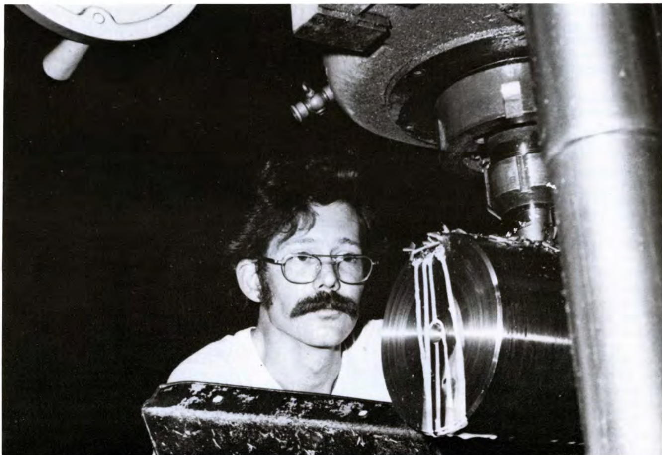
Richard Miller, 2nd shift operator, uses machine #350 in the shaft shop to mill a keyway on a pinion
