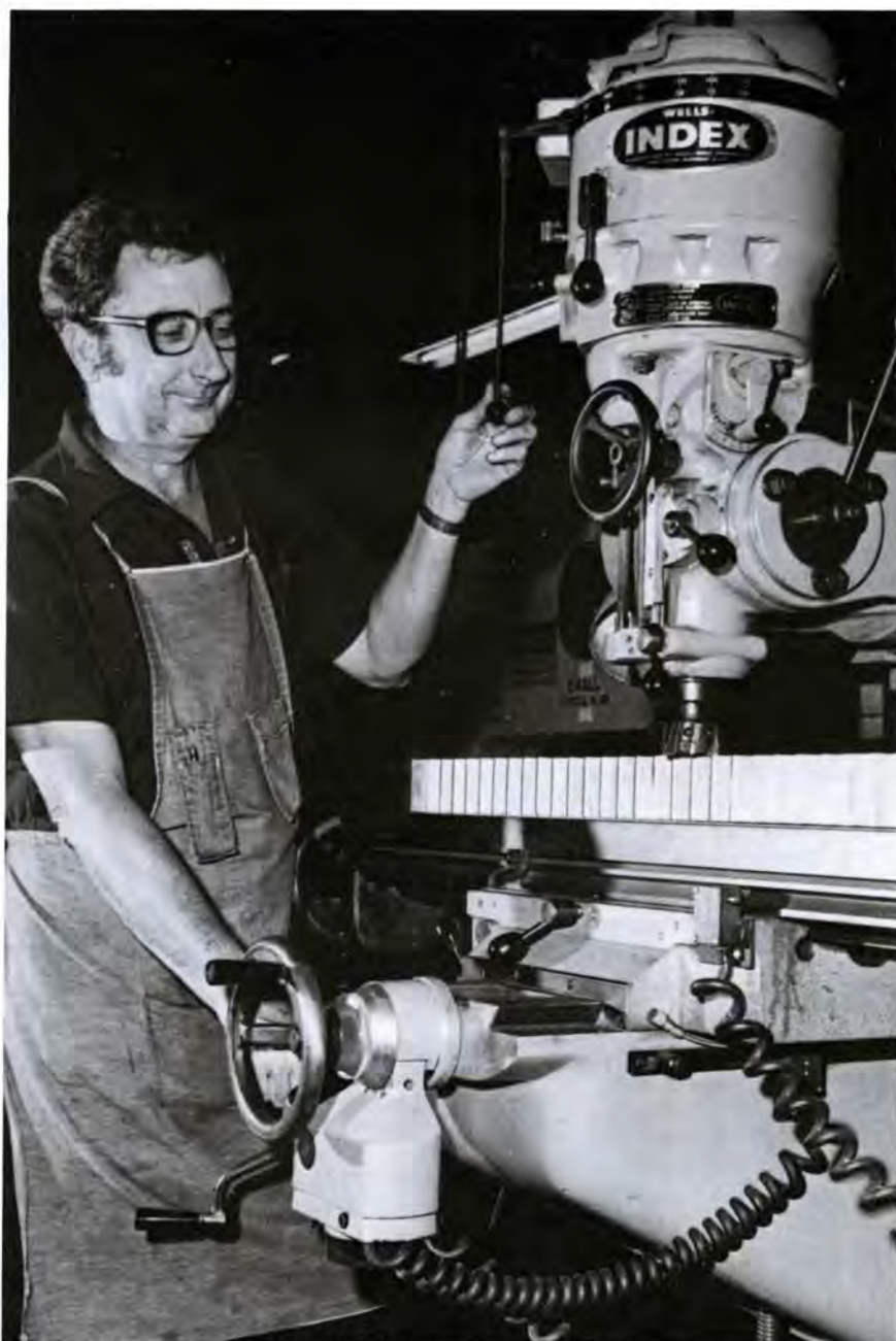
Preston Westbrook, pattern shop, is one of the operators of machine #T-377. Here, Preston uses the variable speed control to mill a pattern
