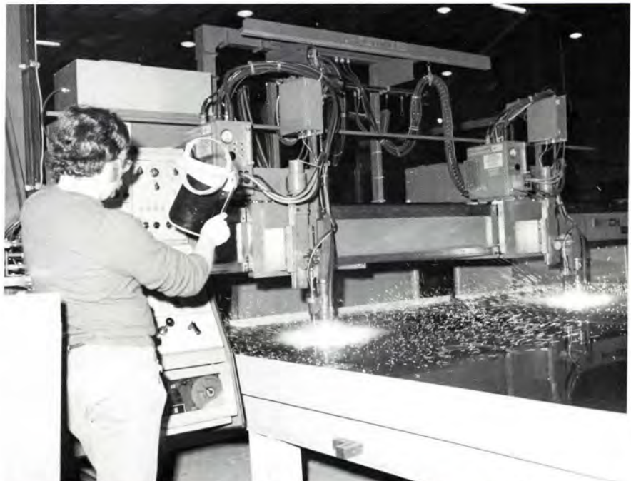
Jim Noullet, principal operator, performs all operator functions at this one location because the control unit is part of the main gantry. This new shape cutting machine is the first computer-operated machine in the welding and structural plant. The control system uses numerical programming similar to the ones used on the machines in the machine shop
