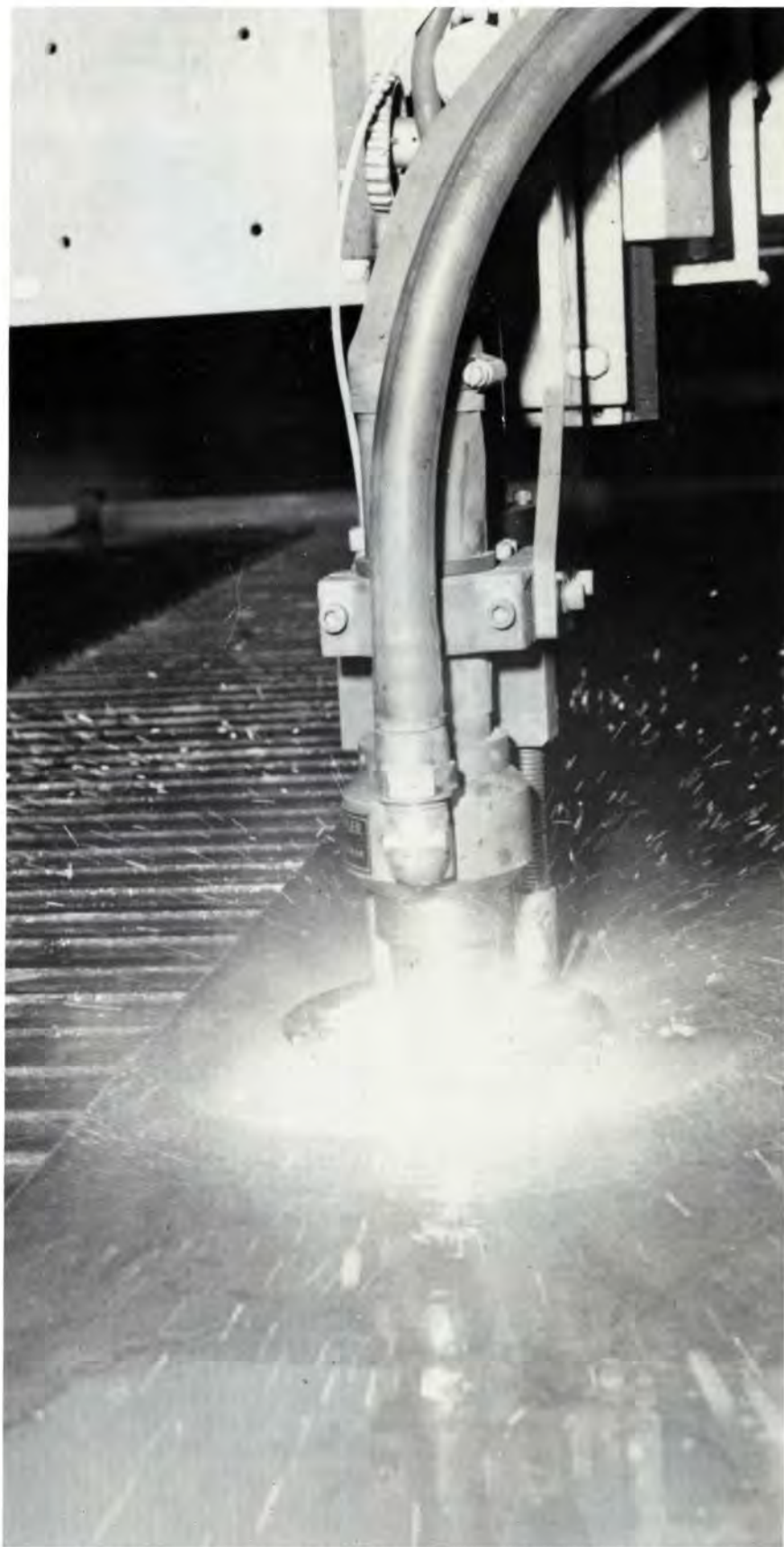
Mounted on the carriage of the gantry are two plasma arc torches. Because of the higher concentration of heat, these torches cut five or six times faster than an oxy-gas torch. Water being injected around the plasma jet further concentrates the cutting arc making it hotter and better defined
