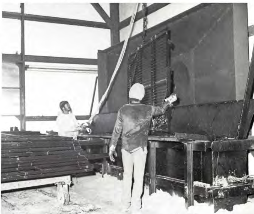
Aaron Henderson, left, and Franklin Clark, both from assembly & shipping, 3rd shift, dip crank guards into a tank which holds 2,750 gallons of paint. The paint is a special one coat combination of primer and black paint which gives a durable protective coating to a set of crank guards
