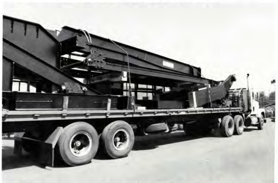
Each part of a pumping unit has a place on the truck bed. Fitting the parts together to make a balanced legal load is the daily job of two teams of men in the assembly and shipping department.
