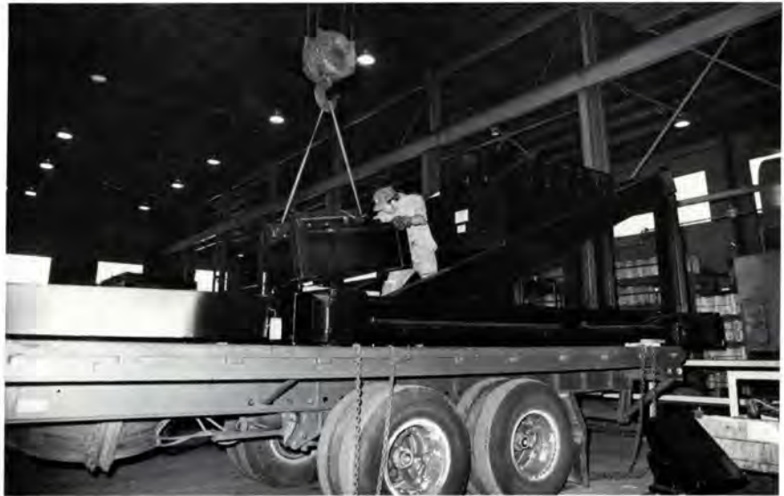
The gear box usually has a standard position on the front of the truck. Jimmy Miller, 1st shift, is setting the motor base assembly in its proper spot on the trailer to insure a safe load. When all parts of the pumping unit have been placed on the trailer bed, a rig has a legal weight on it.
