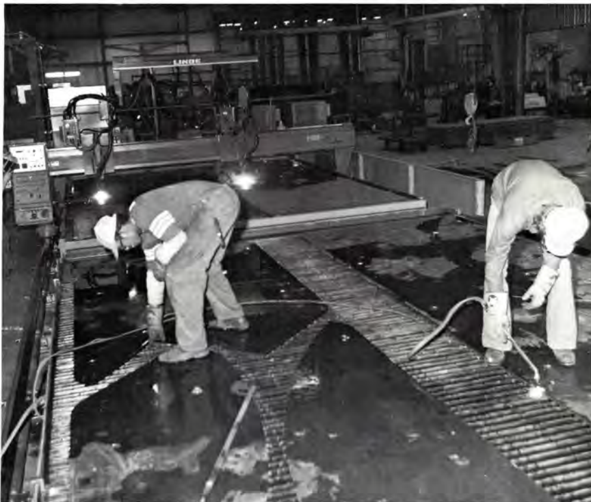
Since the basic machine has a cutting area of 14 feet by 50 feet, material can be loaded or unloaded at one end while material is being cut at the other end. Helpers Eisen Gregory Sanford, left, and Randy Allen, right, cut the scrap away from the horseheads that the shape cutter just finished cutting
