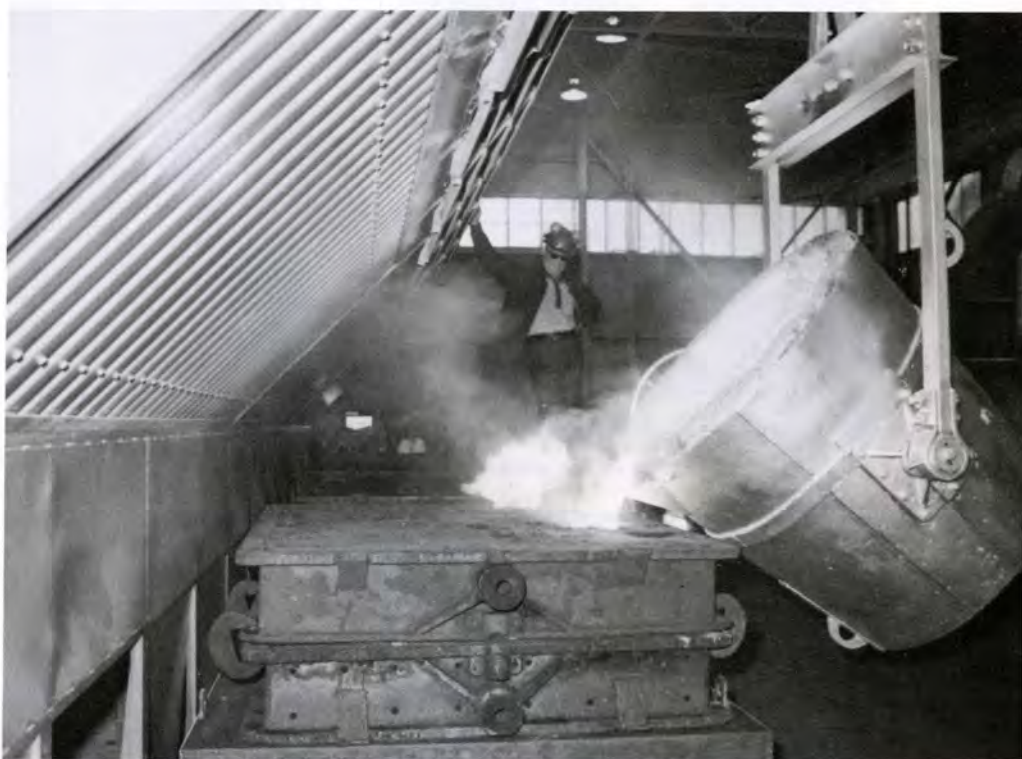
First counterweights are produced as metal is poured into molds
