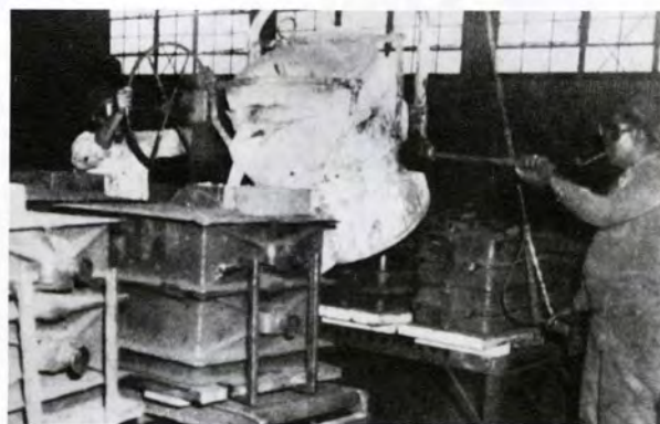
The remainder of the iron would be poured into molds on the side bay, such as these molds for pumping unit saddles.
