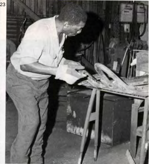
Jim Lewis operates the air hammer that shapes metal for all small parts needed for pumping units and gear units
