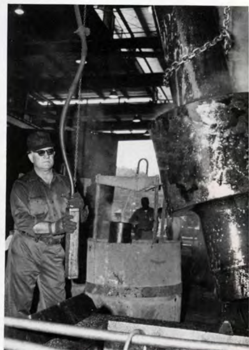
A. C. Lunsford quenches a pinion by placing it into an oil tank. The oil cools the pinion to the desired temperature
