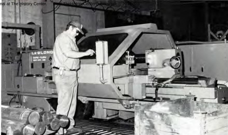
David Frederick, lathe shop, 3rd shift, looks over the new 324 LeBlond numerically (tape) controlled lathe in shaft shop. This machine will be used primarily to produce commercial and marine gears and pinions.
