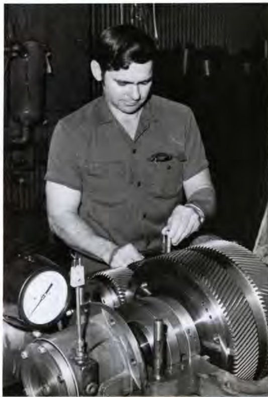
Serviceman Charlie Rhodes inspects tooth contact of a high speed "N" unit which is on the High Speed Gear Test Stand
