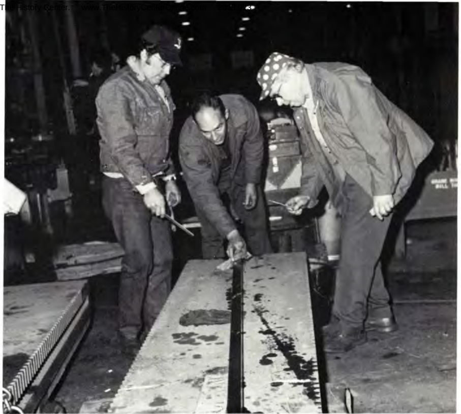
L-r: Joe Powell, Robert Manning, and Kenneth Brashear work on table gib of a crank boring machine
