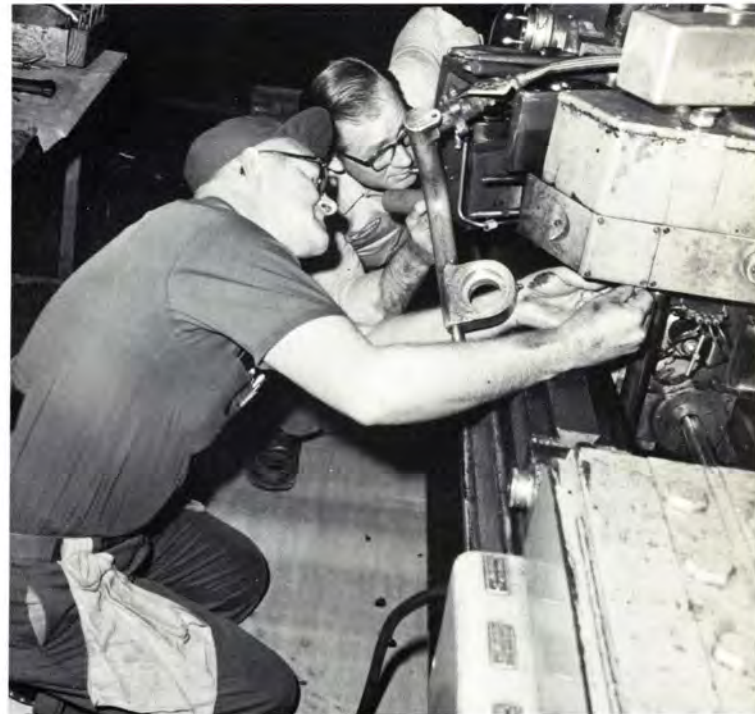
Richard Brashear, (forefront), and James Warren repair tracer lathes, working on carriage and tracer attachments
