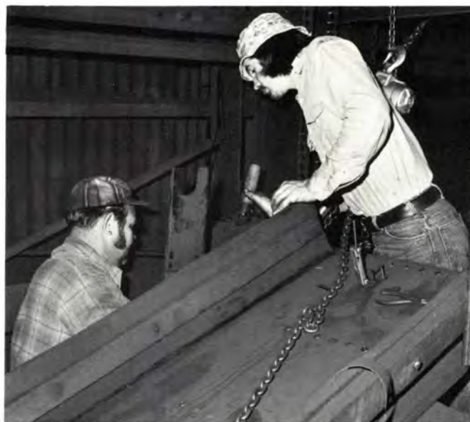
L-r: Roy Tullos and Louis Dunham replace the bearing on magnet of shakeout belt
