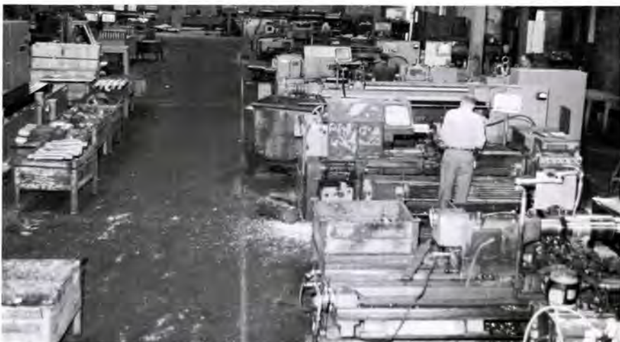
Each of the seven lathes, positioned directly above the underground automated chip handling system, is equipped with an opening in the chip collecting pan. This allows chips and shavings to fall into the conveyor, eliminating shutdown time of the machine
