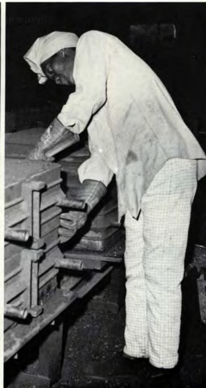
After castings are cooled, clamps holding mold together must be taken off. Alice Thompson (right), shakeout tender, 2nd shift, knocks off the flask clamps before shakeout. After shakeout, Vera Singleton, shakeout tender, 2nd shift, stacks the clamps that have been knocked off the molds so they can be reused the next heat
