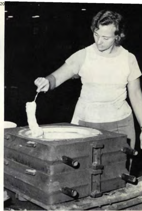
Sue Wagnone, helper in core room, 1st shift, hooks a crane on core which will be fit into a mold. Iron then will be poured in the mold for a pumping unit gear housing
