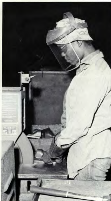
Then castings are sent to Cleaning Room where they are ground by the "chippers and grinders." Ernestine McKelvey (left) uses a floor grinder to clean the "fins" from oil seals and Josephine Patton (right) grinds a bracket. Hand grinders clean hard-to-reach spots on this "box" Lwanda Ligon (center) grinds. All are first shift
