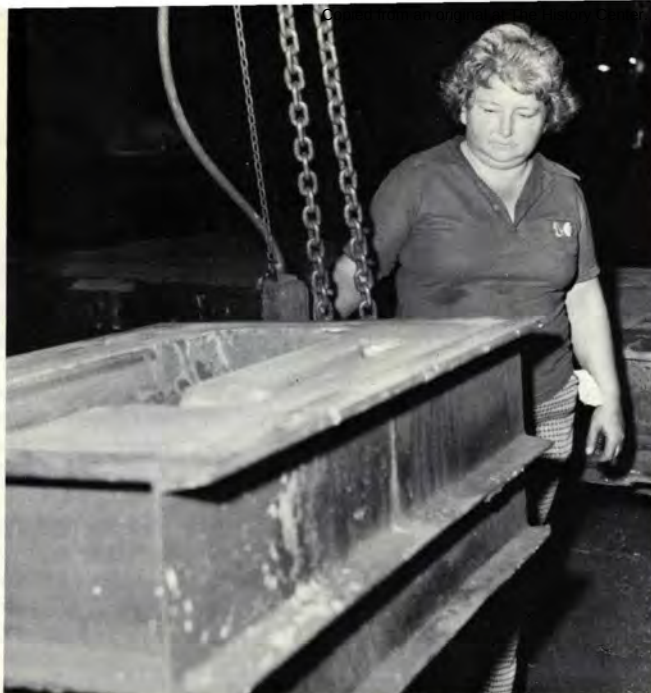
To create a casting with a smooth surface, Georgia Johnson (left) paints mold wash on mold flask, before it is closed. After a mold has been rammed (jolted by a machine to pack sand), it is closed. Dorothy Luman (center) lowers a mold
