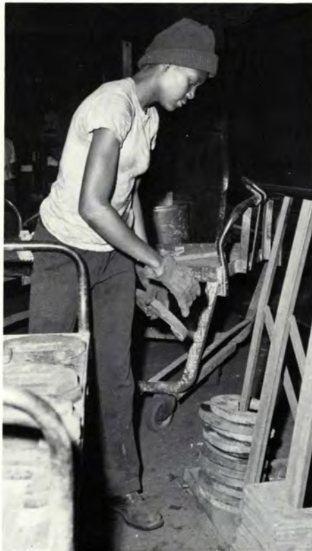
After castings are cooled, clamps holding mold together must be taken off. Alice Thompson (right), shakeout tender, 2nd shift, knocks off the flask clamps before shakeout. After shakeout, Vera Singleton, shakeout tender, 2nd shift, stacks the clamps that have been knocked off the molds so they can be reused the next heat
