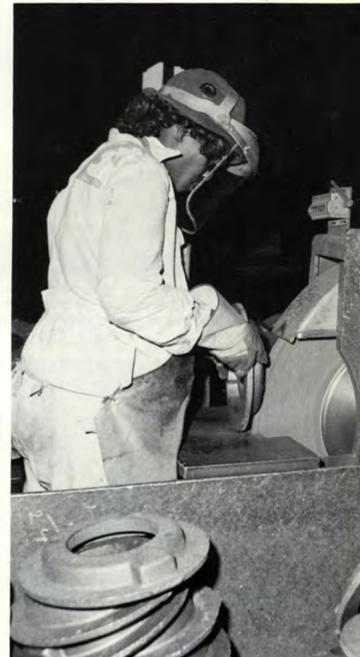
After castings are cooled, clamps holding mold together must be taken off. Alice Thompson (right), shakeout tender, 2nd shift, knocks off the flask clamps before shakeout. After shakeout, Vera Singleton, shakeout tender, 2nd shift, stacks the clamps that have been knocked off the molds so they can be reused the next heat
