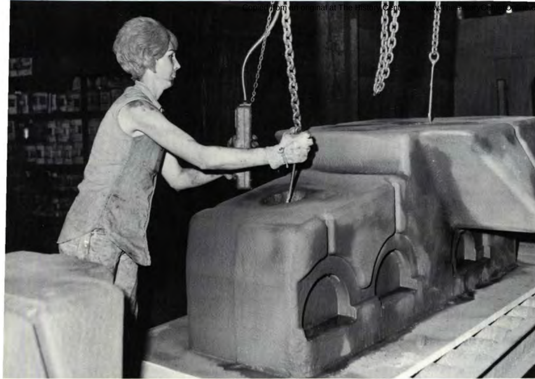
Sue Wagnone, helper in core room, 1st shift, hooks a crane on core which will be fit into a mold. Iron then will be poured in the mold for a pumping unit gear housing
