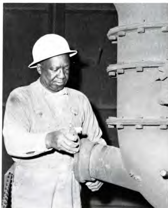
of the six tuyere caps to prevent a draft in the cupola. While burning the bed of coke and sand, air currents, which cause the bed to burn unevenly, are eliminated for a successful "heat"
