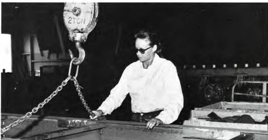
A welder's work is not always welding, as Garvis Edwards has found out. She is helping to turn over an I-beam so that the other side can be welded and finished
