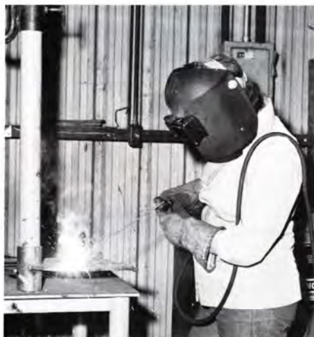
Ethel McClendon, left, shows shielded metal arc welding. Position welding like this is common in all trailer construction
