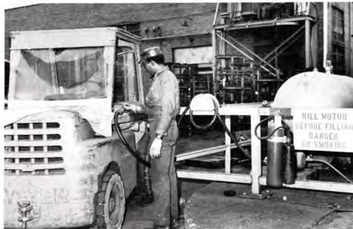
Fork lifts powered by propane engines have proven to be less polluting and more efficient to run. Albert Gilder, Yard Crew, fills up his lift at the propane tank in the Machine Shop yard
