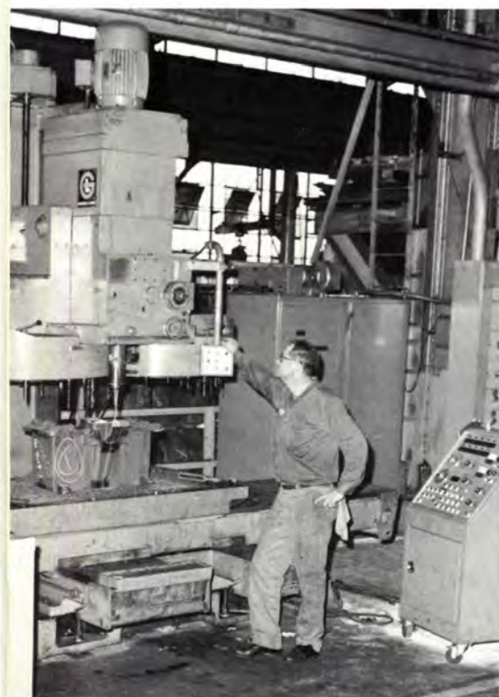
JAMES ELLIOTT on the G&L 310 which has a tool changer that stores and retrieves up to 40 tools in 10 seconds. Primarily, the G&L 310 drills base and parting line holes for speed reducer housings and covers. The G&L 310 and 303 are in the Machine Shop
