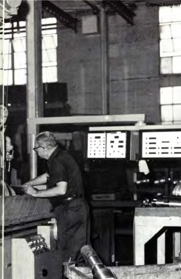
plunge grinding of shaft parts and allows rapid change of as many as eight different diameters, one more addition to Shaft Shop
