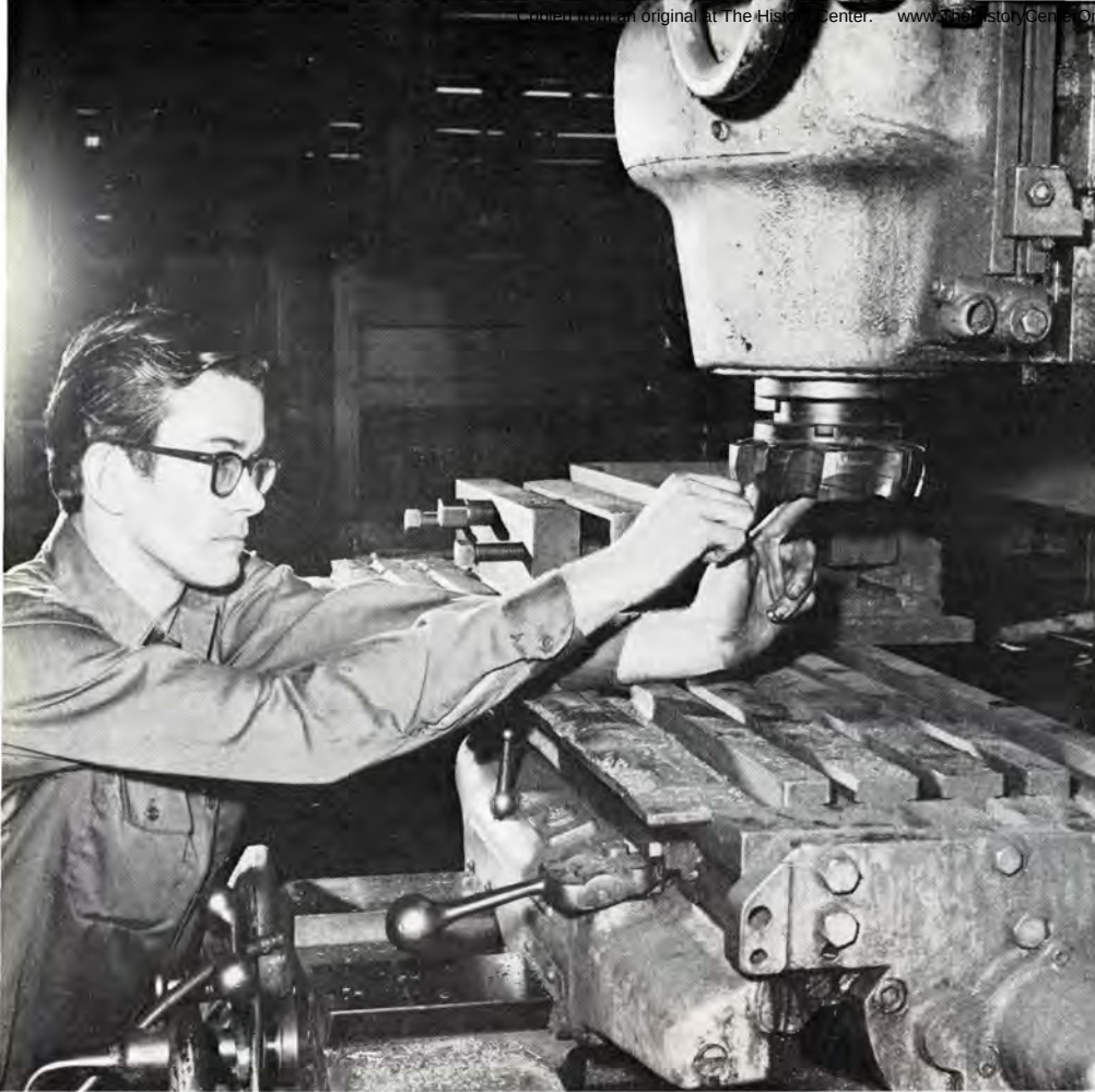
WILLIE is operating a milling machine. He will soon be on a multi-purpose machine which is more sophisticated
