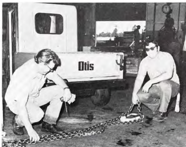
DELBERT ELLISON, left, and Merlin Swan inspect and tag chains to indicate the maximum weight they can transport
