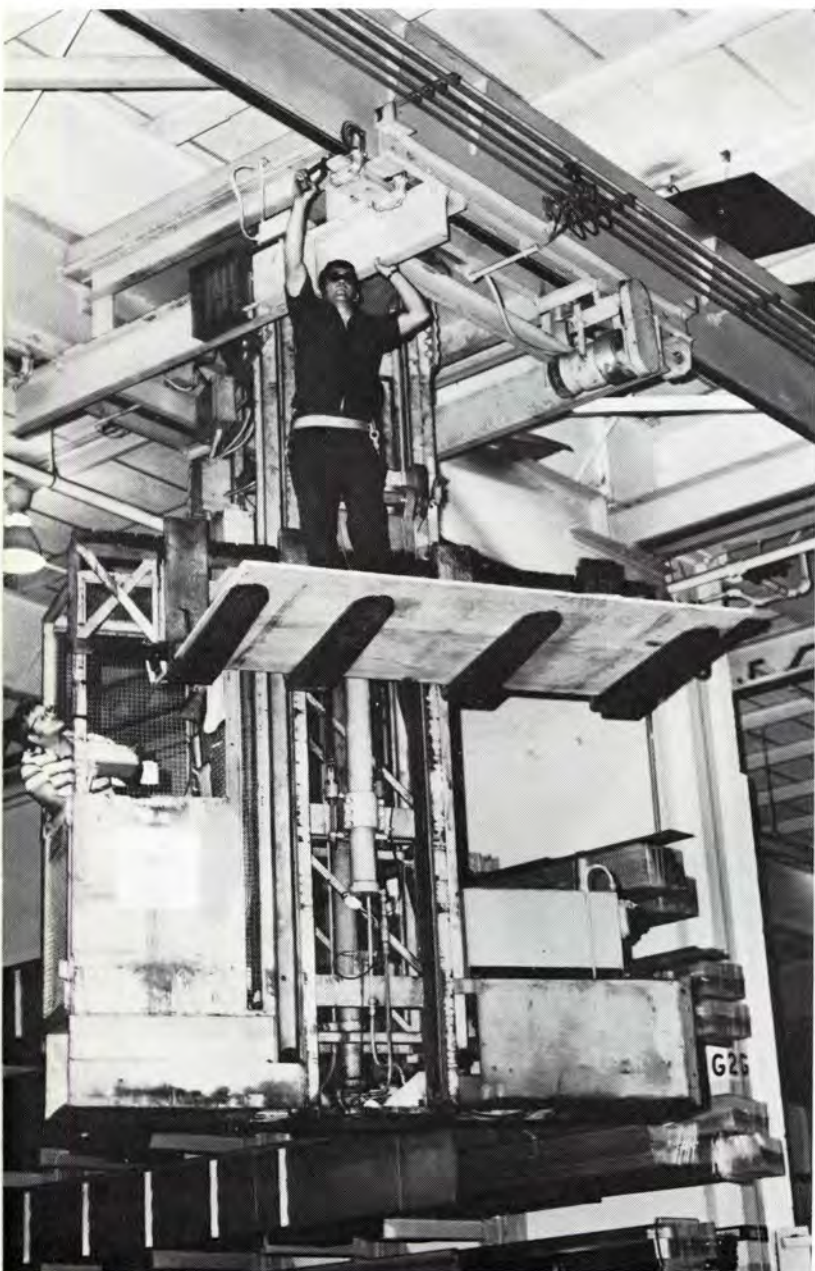
FRED BASEY, mechanic, gets help from Ed Nelson, left, in making repairs on a stacker crane trolley which has broken down
