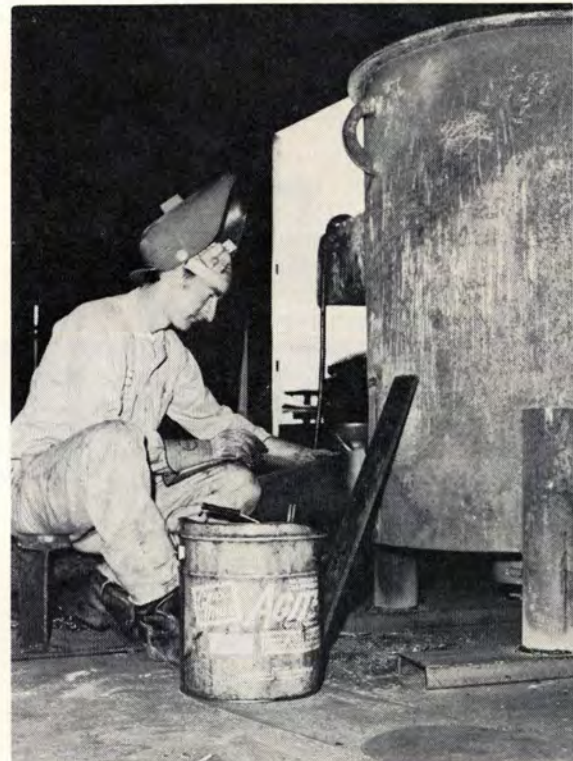
RAYMOND GRIMES repairs a forehearth ladle from the melting department. When he completes the repair, ladle will be returned to its position in front of the cupola for use in the treatment of iron
