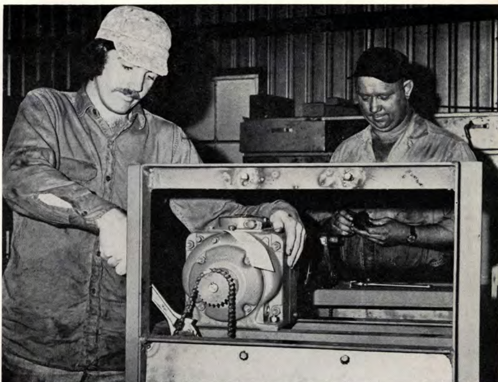
LOUIS DUNHAM, left, and Ray Austin install a resin pump for the no-bake system in the main bay. No-bake has required relatively little maintenance
