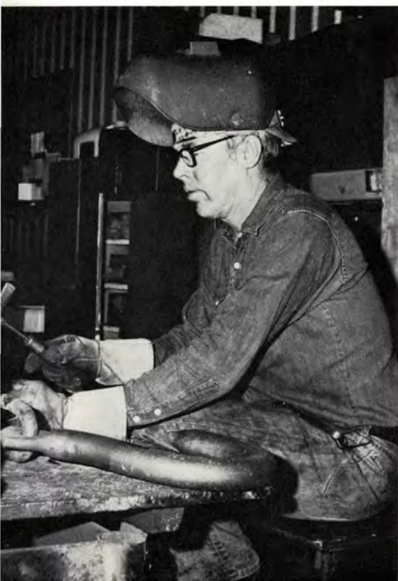
J. C. (BUDDY) JONES welds an overhead crane hook for the main bay
