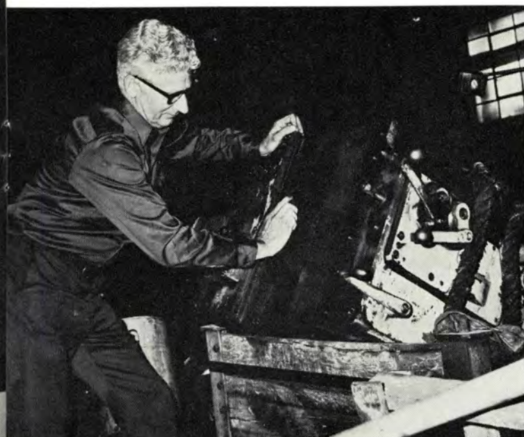
ELTON HENDRY rescrapes and overhauls a milling machine
