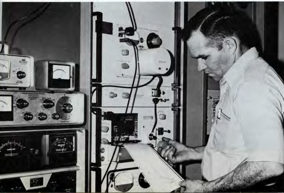
HERE Mike checks the strip chart of a sound test, which is recorded as a graph
