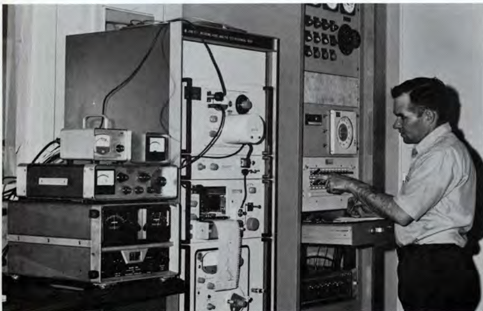
HERE Mike checks the strip chart of a sound test, which is recorded as a graph
