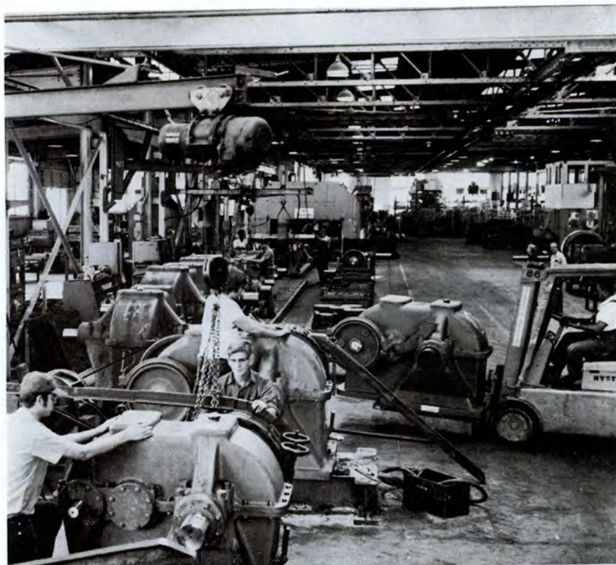
FINAL STEP in quality control is running complete unit on the test block, pictured with Arthur Nelson, left, and Thomas Bone. In immediate background is Mike Conner. Austin Stein is operating fork lift truck. In center background is expanded assembly line conveyor where Malcolm King, Bryan Fox, Leslie Durham and William Curl install both bull gear and high speed gear assemblies, set on cover, fit brakes and generally tighten down unit for transfer to test block. Working at left are William Williams and J. W. Gainer, who are responsible for assembly work on bearing carriers, oil wipers and inspection covers
