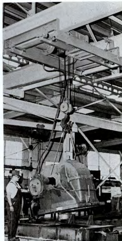
RIGHT: Operating the company's newest crane is Jimmy Freeman, who is moving a completed gear unit from the assembly line to the test block
