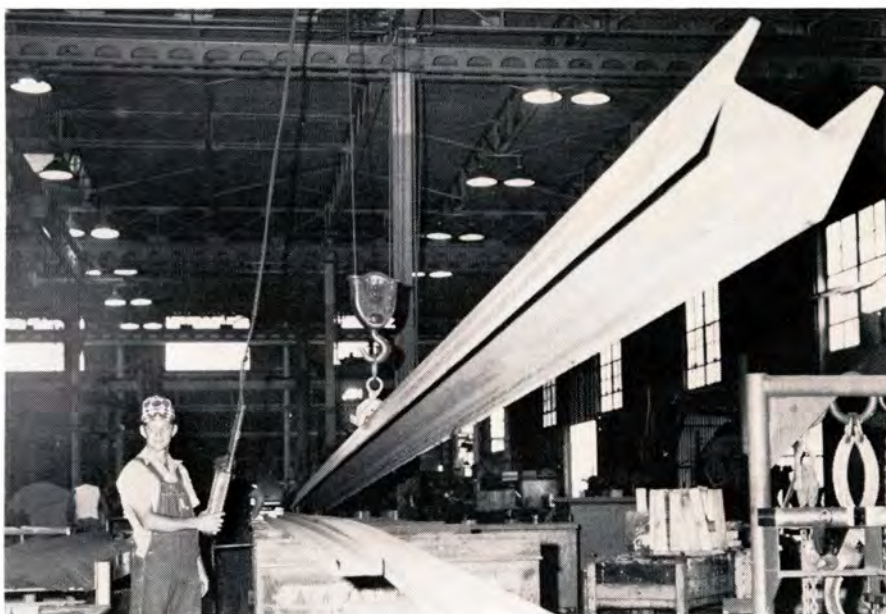
6. J. D. PINNER, second shift, operates a floor-operated overhead crane which is transporting a 49-foot H beam to the DoALL.
