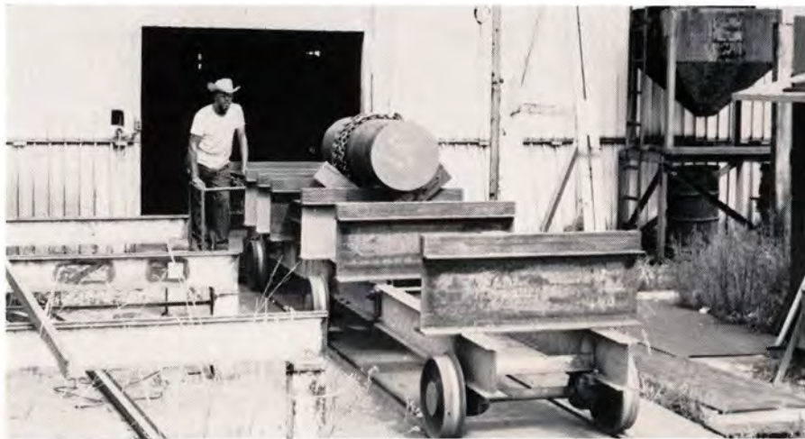
2. BIAS McDANIEL, Material Control, first shift, operates the conveyor car which transports material from the storage yard to the DoALL. The car has an electrically-powered engine which requires less maintenance and eliminates fumes and air pollution.
