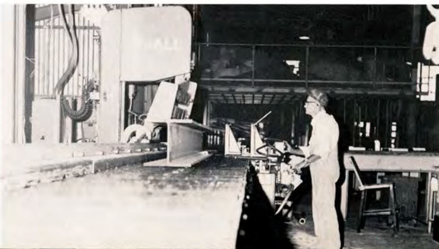
6. J. D. PINNER, second shift, operates a floor-operated overhead crane which is transporting a 49-foot H beam to the DoALL.
