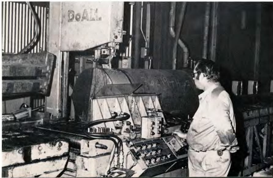
3. AT THE DoALL the round is sawed off to the desired face width for a gear blank. The remainder is transported back to the storage yard. The round pictured, 22½ inches in diameter or 397.40 square inches, was sawed at 8.4 square inches per minute, requiring only 47 minutes of sawing time at the DoALL. R. G. Mitchell, first shift, operates the DoALL. He also records the chemical components and physical properties of the steel used for the customer's verification.
