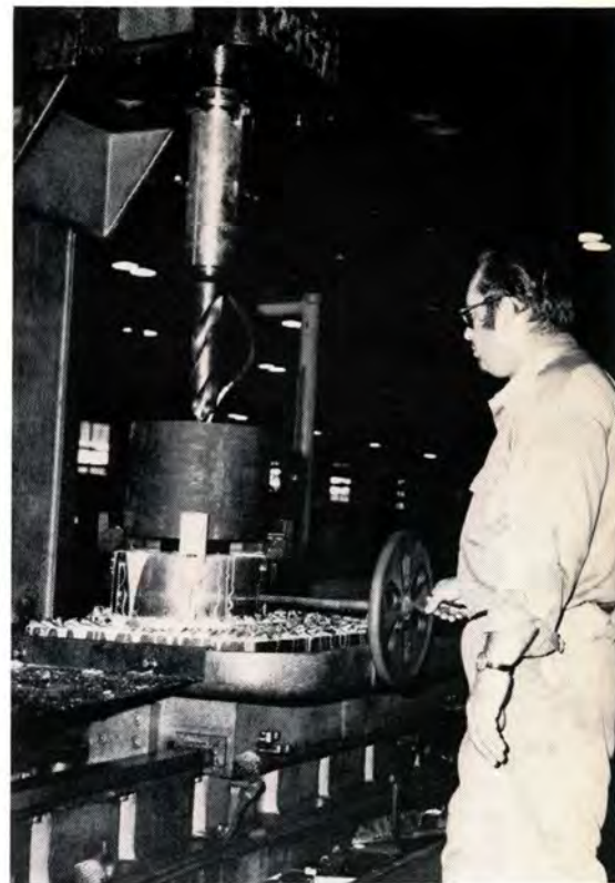
4. THE SHAFT HOLE then is rough-drilled at the nearby vertical drill also operated by Mitchell. From here it goes to the heat treat department, then to the Machine Shop where it is finished turned and bored. Finally it is taken to the Gear Cutters department, where the gear teeth are cut.
