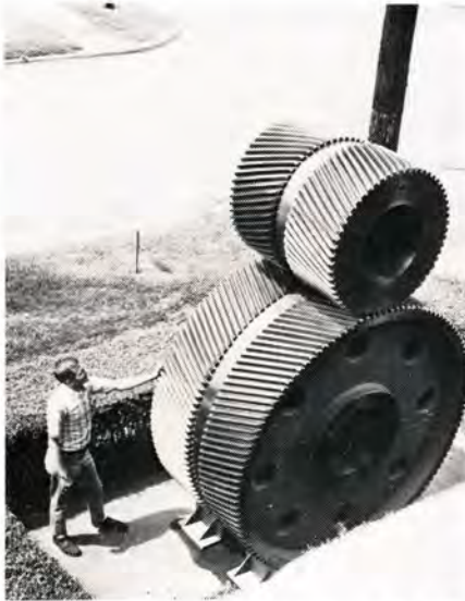
EDDIE SMELLEY, Gear Cutters, first shift, is dwarfed by the low speed gear set mounted in front of the Main Office. Displaying the marine gear unit was his brainchild.
