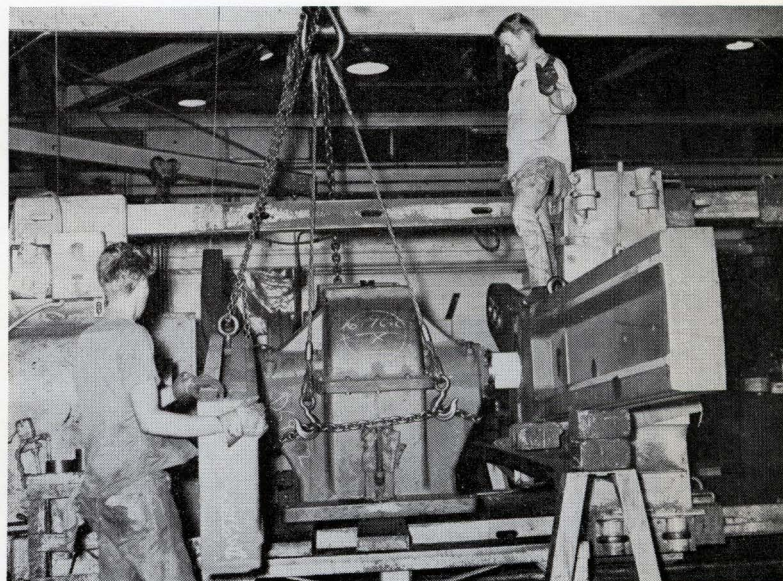
14. SAMMY KIRKLAND directs Larry Shields as the horizontal press presses the crank on the slow speed shaft. The shaft is coated with white lead to prevent galling. Sammy and Larry are employed in the Machine Shop, Assembly Floor, first shift.
