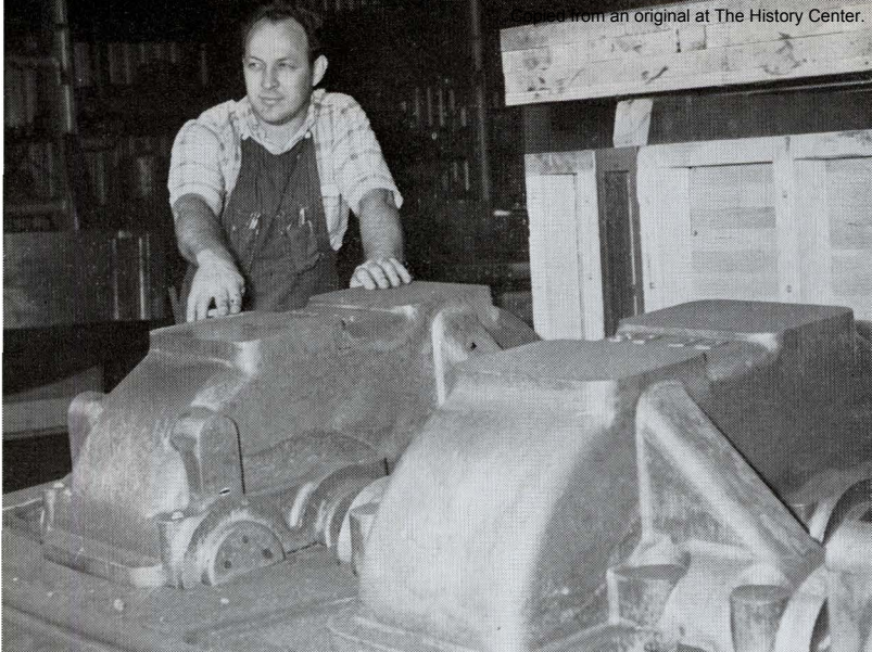
1. SIMULTANEOUS to building the pumping unit's familiar structure, a gear reducer is manufactured.
