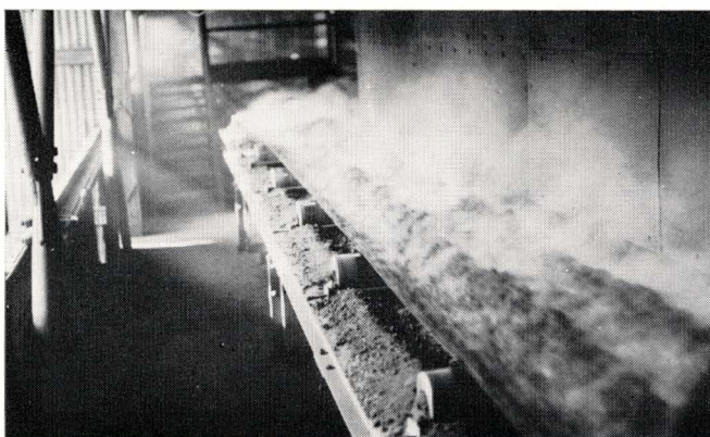
2. IN THE meantime, prepared molding sand is being transported from mullors (sand mixers) to the molding machine. The basic contents of sand used for the keel molds are silica sand, pitch, clay, wood flour and water.
