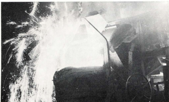
6. FROM the holding ladle the metal is transferred to the pouring ladle, which has a capacity of 11,000 pounds. At this point in the process, magnesium alloys are added to convert the base iron to ductile iron, a stronger, more durable material.
