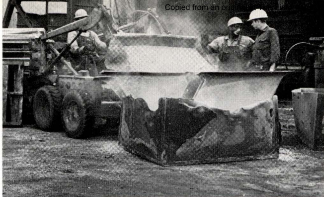
11. HERE the keel is packed with gravel in a heat treating pan. Left to right are Chester Robinson, Early Mathis and Ralph Jones.
