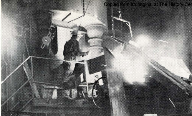
5. MOLTEN iron emerges from the cupola at a temperature of 2600 degrees. During this "tapping out" process, the liquid metal runs down a trough to the holding ladle. Seamon Rigsby taps the hole.
