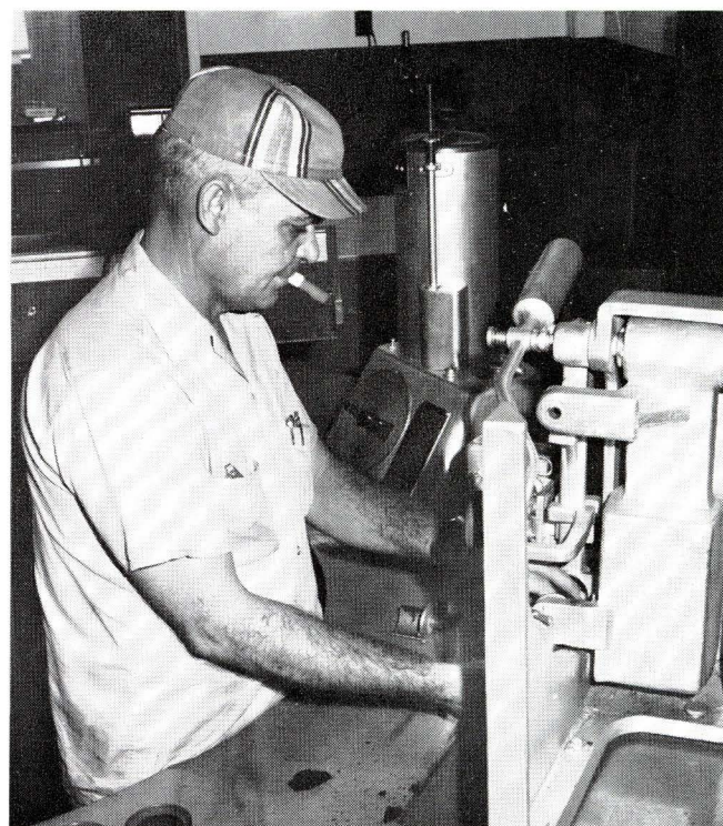
PHILLIP SHARP puts a sample on the green strength machine to see if it has the proper strength.
