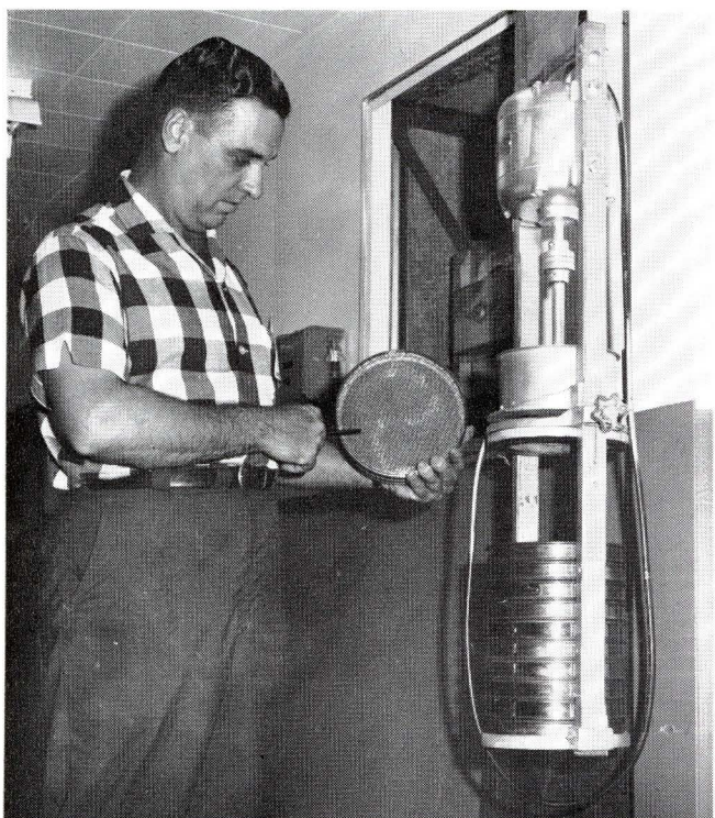
FRANK MARTIN shows how the fineness of the mesh varies on the Gyratory Screen.
