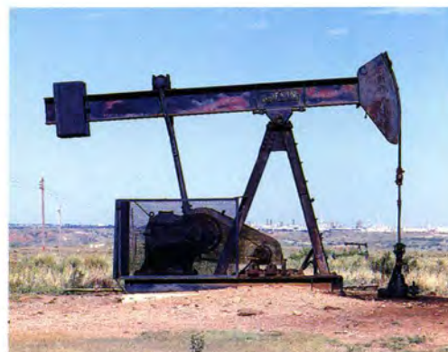
LUFKIN SC11A, Phillips Petroleum Company, Cockrell Ranch, Well No. 22, Borger, Texas. One of many LUFKIN pumping units still in operation after nearly 50 years of service.
