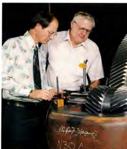
Assisted by Louis Lloyd, project engineer, Leonard Avery, right, manager of LUFKIN's gear service department and high speed test supervisor, inspects the vibration probe shaft area of a N3004C Gear Reducer for electrical and mechanical run-out.
