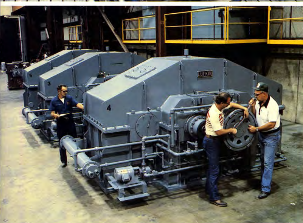
(Above), Testing of high speed gearing is also handled by the service department. Here, service representative Kyle Syler prepares a unit for testing. (Below), (l-r) Service representatives Ken Crawford, Chuck Anderson and David Massingill make a final inspection of one of the large TC-4824 sugar mill gears in for repairs.
