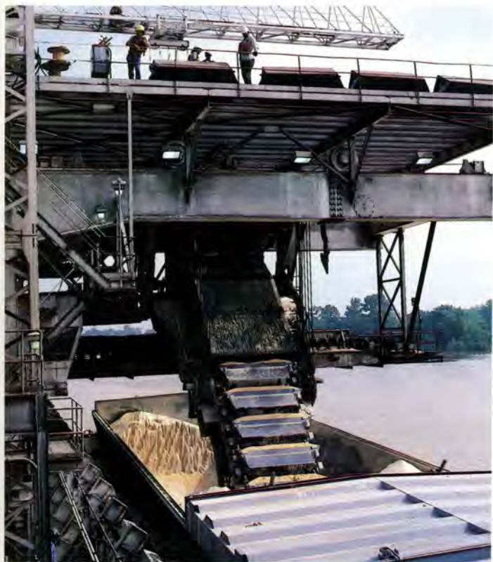
(far left) The K-2 mid-stream bulk transfer rig is mounted on a hull 330 feet long and 75 feet wide. (middle) The trolley rack drive for the unloading system is driven through a LUFKIN T195C Gear Reducer. (left) The bucket drive which empties bulk commodities from barges utilizes a LUFKIN THB440C triple reduction right angle gear.
