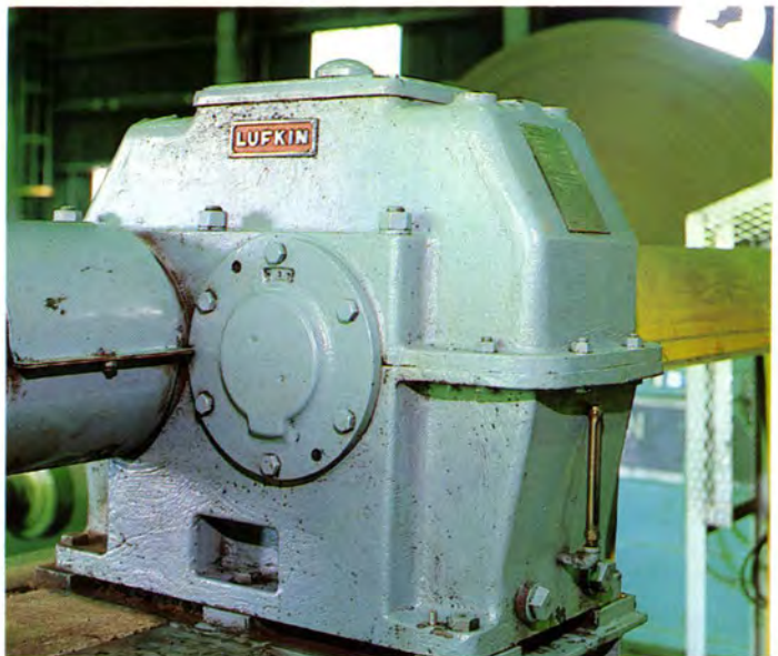
A LUFKIN S127C Gear Reducer is driven by an electric motor at 1,750 RPM that powers a paper machine reel located in an Ohio mill operated by Stone Container Corporation.
