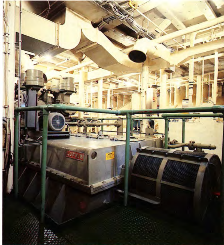
The "Surry," a ferryboat operated by the Virginia Transportation and Highways Department, is powered by a 1,450 HP EMD engine through a LUFKIN RHS2613S Reverse Reduction Marine Gear. The unit features a unique single input and dual output arrangement.
