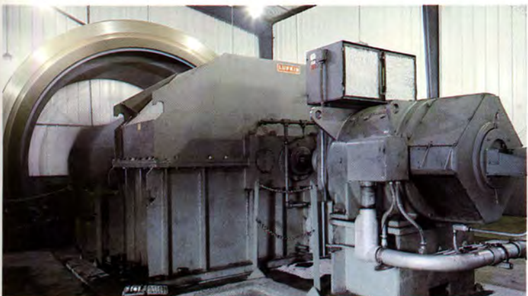
A LUFKIN DF780C Industrial Gear Reducer transmits 400 HP at 400 RPM to a coal hoist drive in a West Virginia coal mine.
