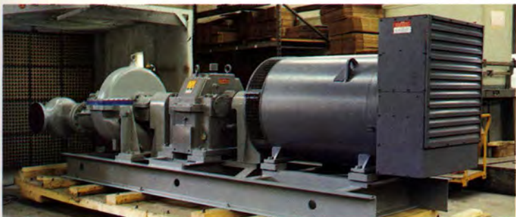
A LUFKIN N1002C Gear Reducer is driven by a turbine at 4,000 RPM to a centrifugal pump at 1,168 RPM.
